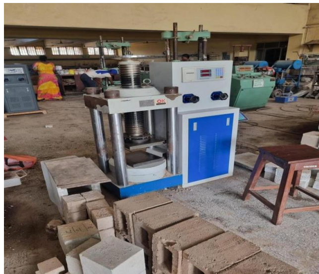
Fig 1: Universal Testing Machine (UTM)
