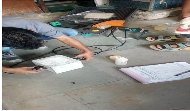
Fig 4: Experimental setup to perform ultrasonic pulse velocity test (Actual photograph of the setup)
